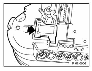
Insert encoding connector and clip in new retaining frame.
